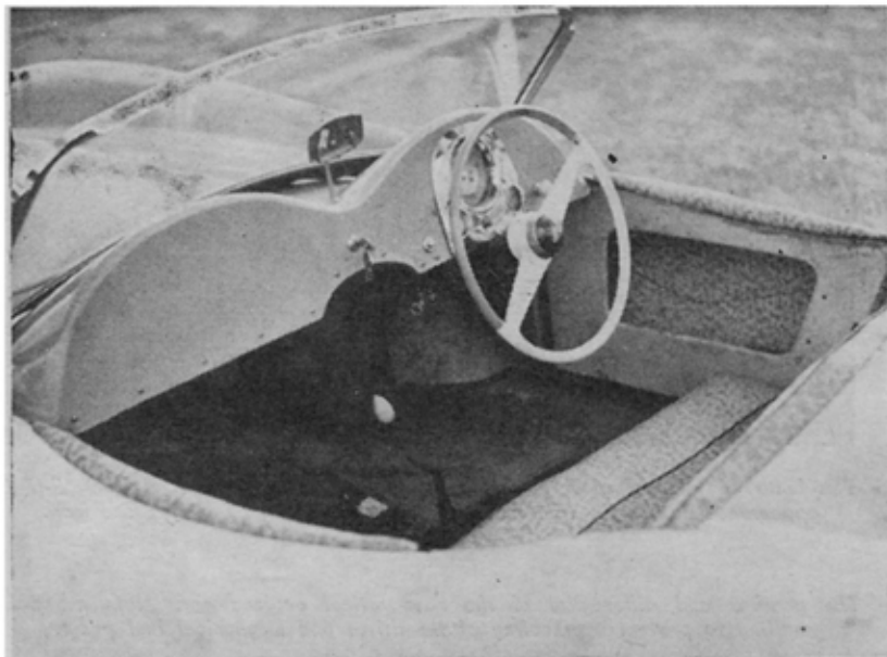
Cockpit of the Holden is spartan, utilises Holden components wherever possible. All the running gear is Holden, some stock, some modified.
