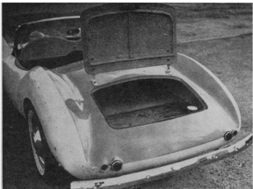
The body of the Holden special is quite well finished, has largish luggage locker, which also accommodates fuel filler.
